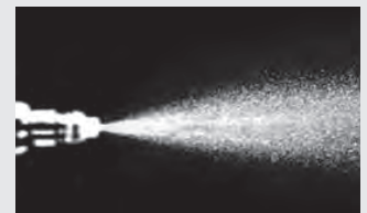
Injector spray pattern after P.i. treatment.
