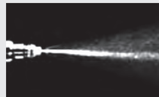
Injector spray pattern before P.i. treatment.
